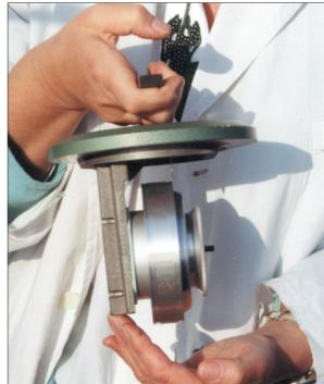
Fig. 2. 7-day volumetric trap
