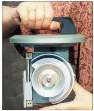
Fig. 3. 24-hours volumetric trap
