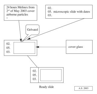
**Fig. 4.** Schematic diagram of laboratory preparing slide with diurnal record of airborne particles
